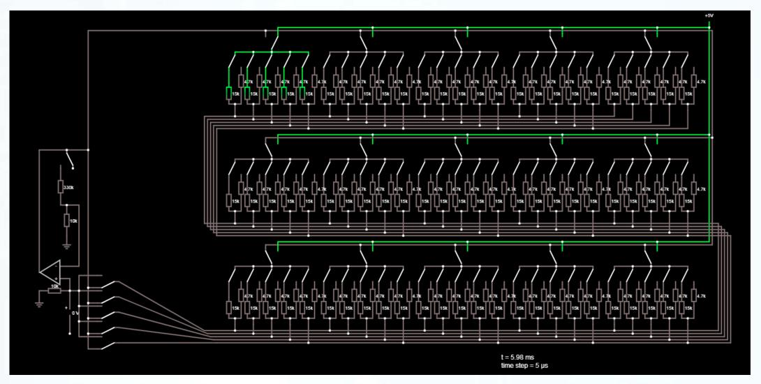
Despite greatly reduced wiring requirements, it is still a necessity to multiplex microprocessor outputs to achieve the 20 I/O connections needed.
